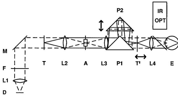
Fig. 1. Schematic of the Badal optical system for stimulating accommodation of the eye (E). Dashed lines show the optical path from the source of illumination, and solid lines represent target optics. Interference filters of three bandwidths (10, 40, and 80 nm) could be introduced at F to alter the spectral composition of a square-wave grating target (T). The sinusoidal motion of prism P2 moved an aerial image of target T' toward and away from the Badal lens (L4) through a range of 1.0 D.
