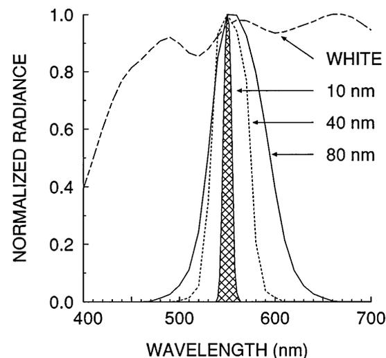
Fig. 2. Spectral distributions of the four test conditions (10, 40, and 80 nm and white) normalized to their individual peaks. The bandwidths specified here are nominal in that they refer to the filter manufacturer's specifications of bandwidth at half-peak transmittance.
