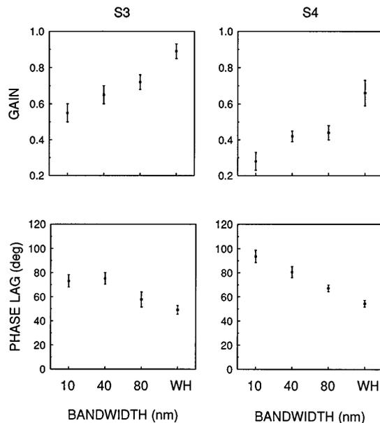
Fig. 4. Gain and phase lag of accommodation as a function of the spectral bandwidth of the target for two typical subjects, determined by a vector average of five trials per condition. The gain is an amplitude ratio (response/stimulus), and the phase lag is a time lag of the response with regard to the stimulus. As the target's spectral bandwidth increases, accommodative gain improves and phase lag declines.
