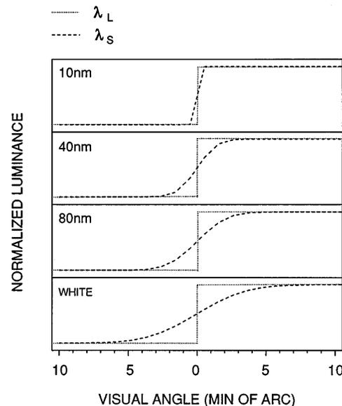
Fig. 7. Effect of increasing spectral bandwidth on the blur-spread function (of a luminance edge) for an eye with a 4-mm pupil. The longer wavelength ( $\lambda_L$ ) of each spectral condition is in focus (dotted curves), and the shorter wavelength ( $\lambda_S$ ) is out of focus (dashed curves) by an amount dependent on the longitudinal chromatic aberration produced by light of these two wavelengths.
